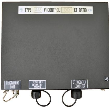
For applications with high humidity, the possibility of flooding, or where submersion is possible, G&W provides a Type 4.1 control in an IP68 rated enclosure which is fully sealed with epoxy compound and is rated for 20 days of submersion under 20' of water.
