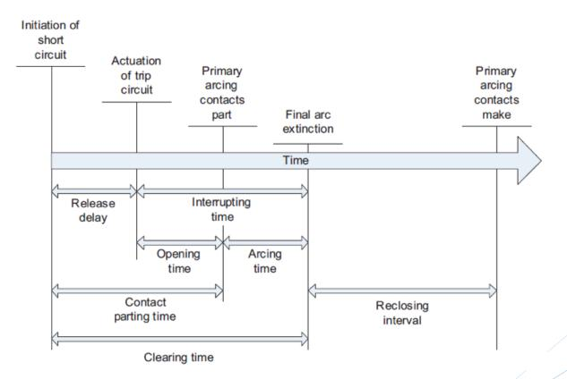
Figure 1: Graphical representation of Clearing Time
